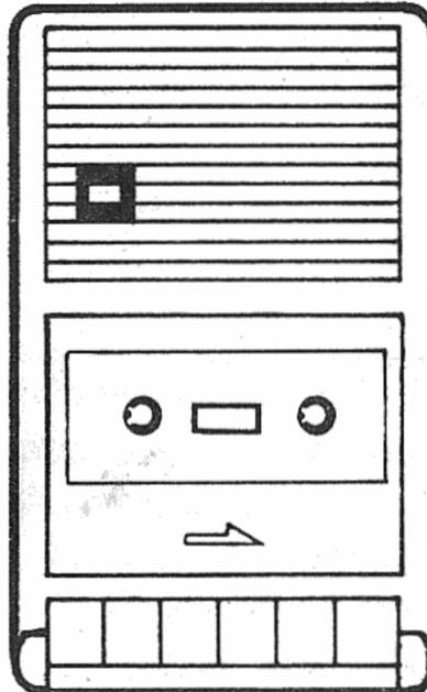
4. Key the CLOAD command. As soon as you do so, the recorded program will begin to load into the computer system, and the screen will list this program.
